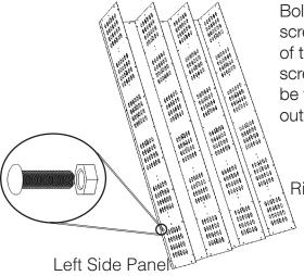
Bolt the tamper-proof screw on the inside of the locker. Only the screw heads should be visible from the outside of the locker.
