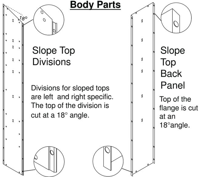
Bottom of divisions and back panels have the first hole on flange 1-3/4" from edge, (top of divisions and back panel have the first hole 1-1/4" from edge).
