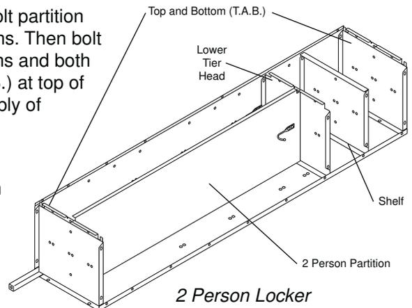
Single row lockers must be floor and wall anchored,
