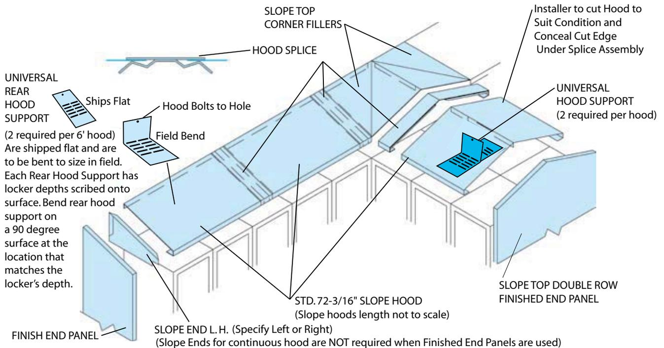
Single row lockers must be floor and wall anchored, double row lockers must be floor anchored and if possible wall or ceiling anchored.
